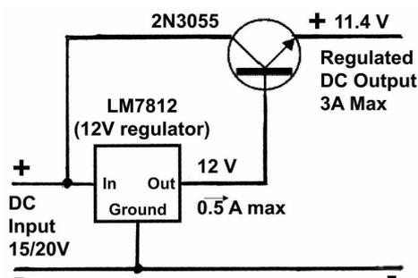
**Note:** Although the regulator outputs 12V to the base of the pass transistor, there is a 0.6V drop (on average) from base to emitter. The output voltage equals the regulator output minus 0.6V for every base/emitter junction in series with the path to the output terminals – in this case 11.4V. Here, the regulator is grounded.
