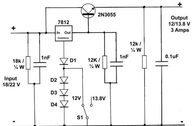
By putting a resistor across the input and the output of the regulator so that 1 or 2 mA is drawn, a DC "path" is provided for the internals of the regulator. The 1nF capacitors across the input/ output of the regulator act to help reduce RF interference.
