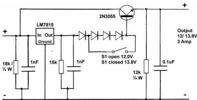
The regulator will produce 15V. The output voltage of the complete circuit will therefore be 15.0V, less 0.6V in the pass transistor (TR3), less 0.6V for every series diode. Therefore, to achieve 12.0V output, 4 diodes are needed in circuit. To achieve 13.8V, 1 diode is required.
