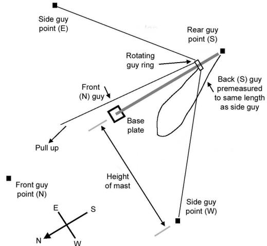
Fig 8.1a - Basic guying arrangement for simple small mast (plan view)
