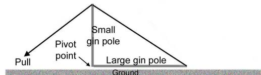
Fig 8.3a: Using a small gin pole to raise a larger one
