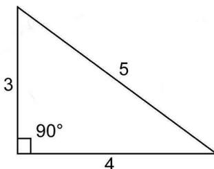
Fig 8.1c: 3, 4, 5 triangle as used for setting out ropes at a right angle (90 degrees)
