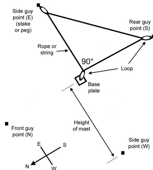
Fig 8.1 c: Arrangement recommended by G3ZMF for accurately setting out guying points
