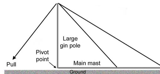
Fig 8.3b: Subsequently using the larger gin pole to raise the main mast
