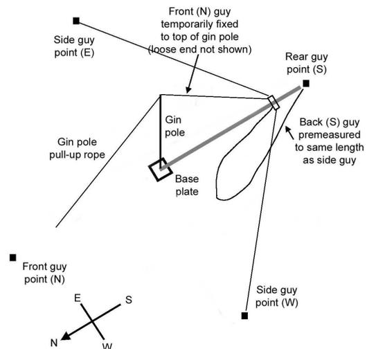
Fig 8.2 a: Using a gin pole (falling derrick) to raise a large mast. Note that for simplicity only one set of guys is shown here: in practice two sets would be advisable, one set attached to the top of the mast arrangement and the other around halfway up. Also, for simplicity, additional gin guying is not shown but may be needed for a large installation.
