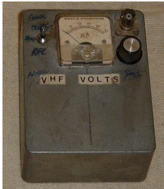
External view of G3ZMF's all-purpose sniffer
