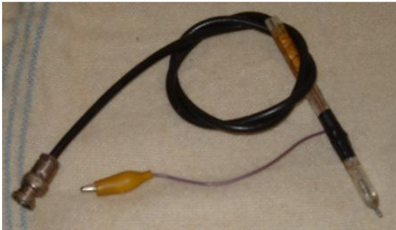
Probe 3: A coax lead with a probe constructed from an old ball point pen case.
