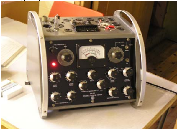
G4FKK's AVO Mk.3 valve characteristic meter
