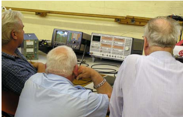
At work testing a members' kit. The test gear is a Marconi 2955A and a Rohde & Schwartz CMT55 multi-function RF analysers
