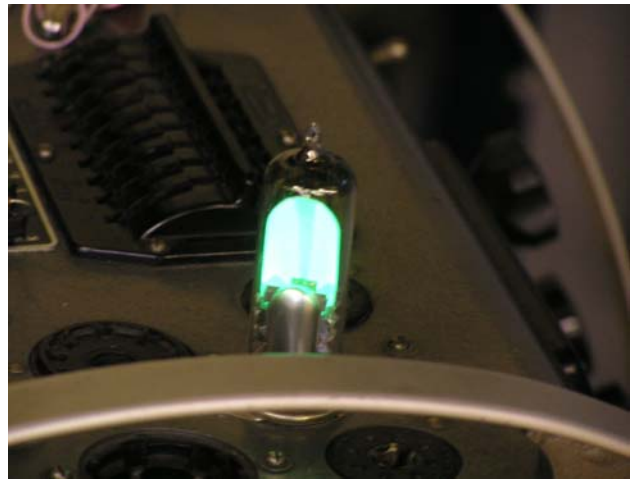
Successful test on an EM81 "magic eye" indicator
