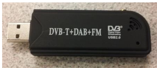
A TV dongle of the type that could form the basis of an SDR (software defined radio) when use with a Raspberry Pi
