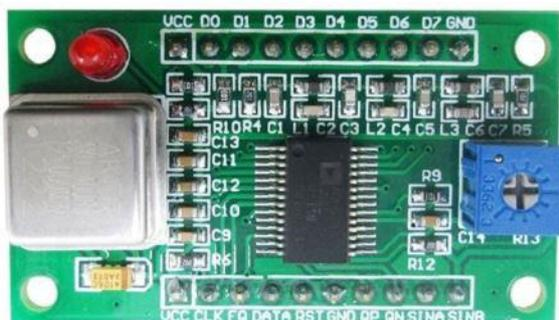
An AD9850 DDS Signal Generator Module
