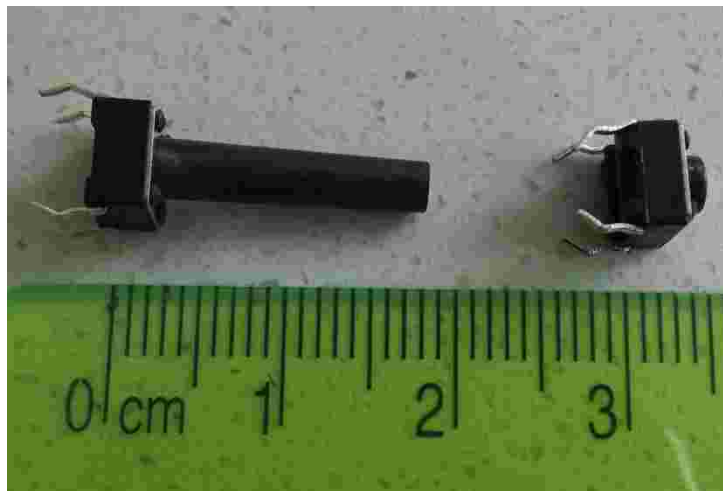
Tactile Buttons: L – as installed by G3WZK; R – as supplied in the Adafruit kit
