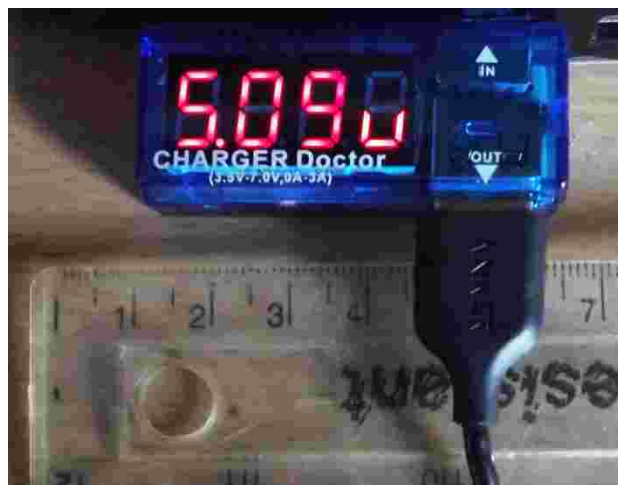
The “Charger Doctor” In Use at G3WZK – indicating that its input voltage is 5.09 volts
