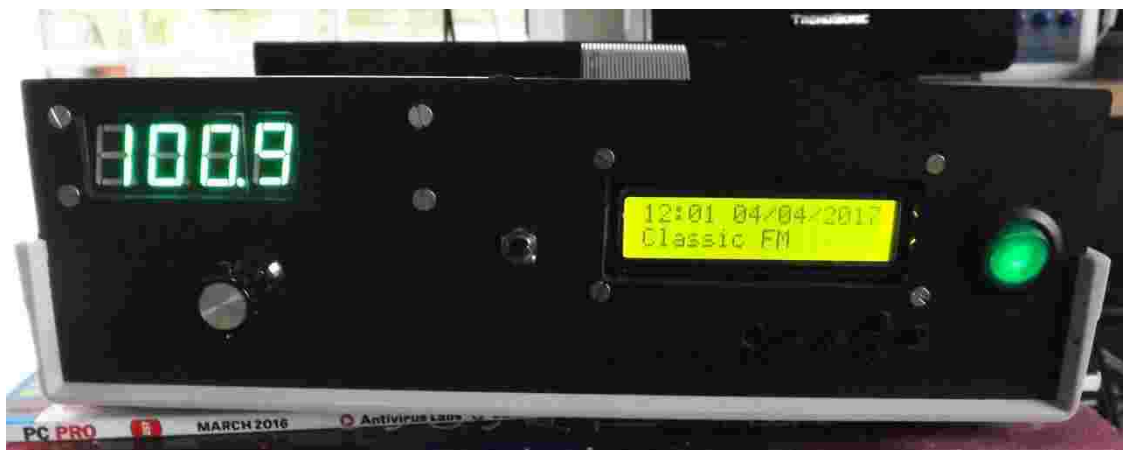
The completed dual VHF/RaspberryPi radio under test, but before applying any labels to the front panel. Classic FM is being received on VHF (left hand radio) and also via the Internet (right hand radio.)
