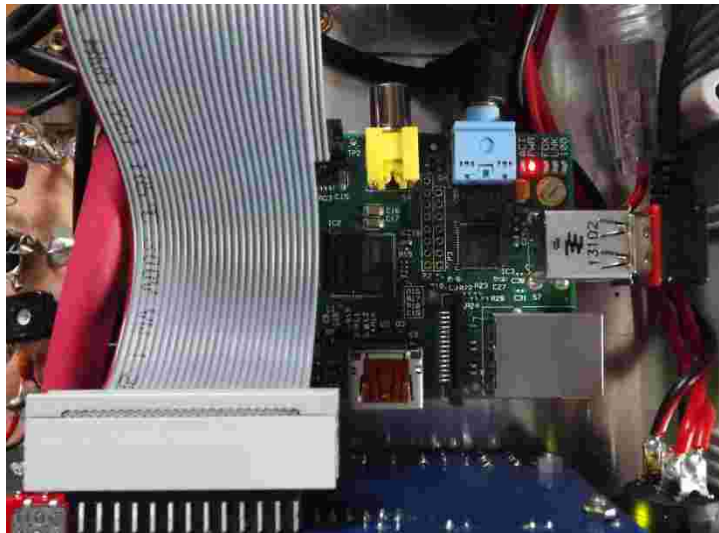
The RPi Internet Radio installed in the radio box – Wi-Fi dongle at right
