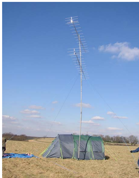
The 2 x 2m stacked Yagis towering over the CATS tent
