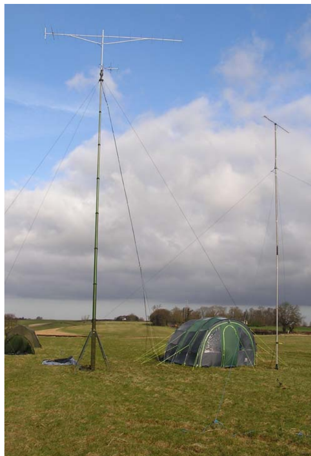
The main 2 metre antenna on the main mast with the 70cm antenna next to it. The small 3-ele antenna just above the rotator was used as a wider beamwidth "search" antenna.
