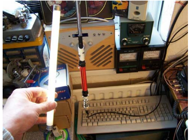
Pic 6. A mere 2.5W can light a fluorescent tube at some distance!
