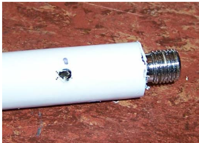
Pic 2. 3/8" fitting atop the loading coil
