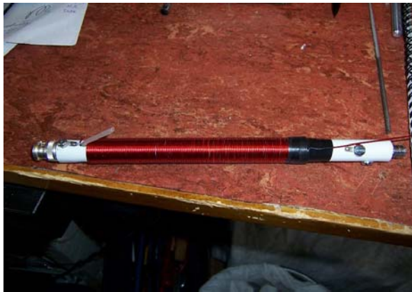
Pic 4. 125 turns of 1mm dia ECW.
