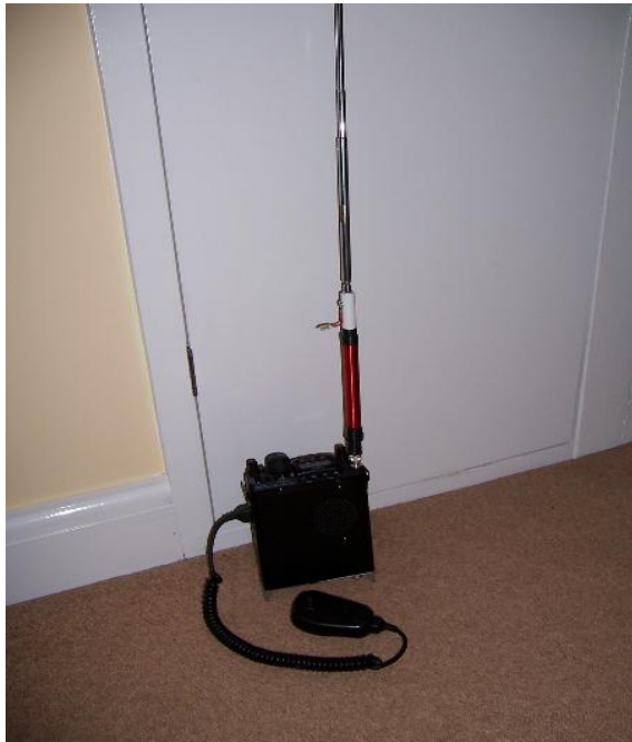
Pic 7. The whip a-top the rig
