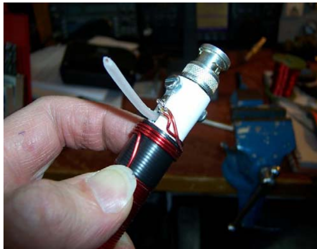
Pic 3. The coupling coil and BNC plug at the base of the coil
