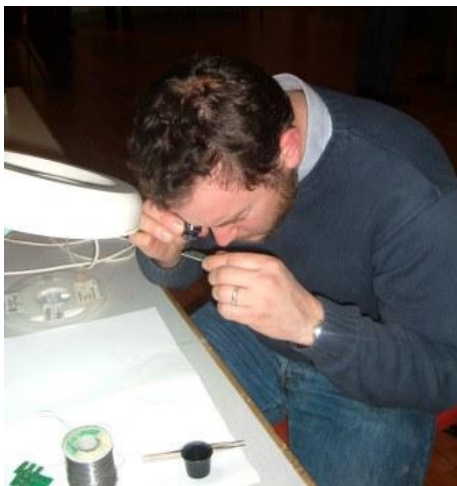
Paul, 2E0JXN, checks out his SMD board for dry joints
