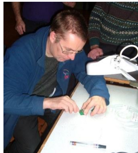
Dennis, M0NDJ, prepares to solder in his first SMD. Note flux pen in the foreground
