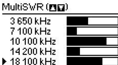
Simultaneous measurement on different frequencies – bar chart display
