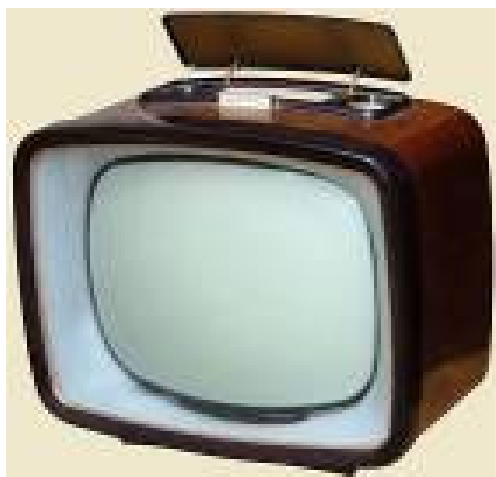
The old Murphy TV – all user controls were under the flap that opened in the top of the set
