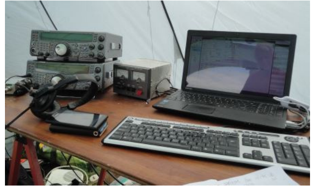
Double decker TS-2000 -Mine at the bottom with autocalling but only 18 watts, and Stuart's on top capable of transmitting the full 25 watts required
