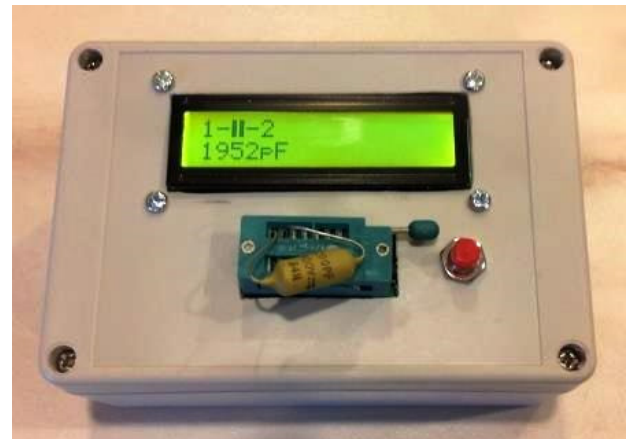
The completed and boxed-up project. Note the red push-button that is wired in parallel with the original PCB-mounted test button.
