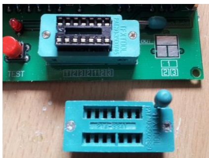
The PCB with the 14 pin DIL IC socket in place, ready for mounting the second latching socket.
