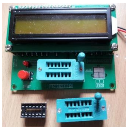
The additional sockets ready for insertion
