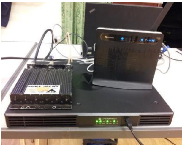
DMR equipment that Denis G0OLX brought to the meeting. On the left side is a PA (power amplifier) unit. On the right (with the blue LEDs) is a 4G router used to provide internet access. Both items are sitting on the DMR repeater (with the green LEDs.)
